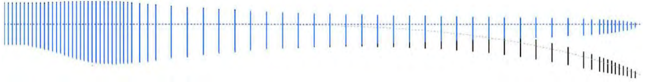
Figure 4: Discretised model of the straight and the swept blade [5]
