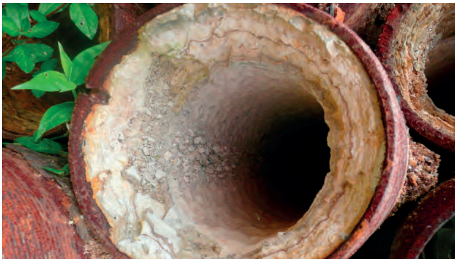
Fig. 17: Plant components at an Indonesian geothermal power plant showing massive silica precipitation (scaling) and a significantly reduced cross-sectional area available for flow.
