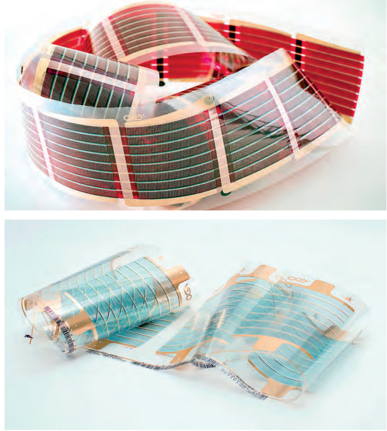
Fig. 4: Solution processed organic photovoltaic module (top) and a transparent conductive substrate separately (bottom). Picture source: [2]
