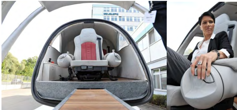
Fig. 11. Sphere sidesticks integrated in the driver's seat
