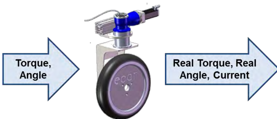
Fig. 7. eCorner as highly integrated smart component.
