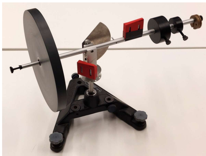
Fig. 1. Gyroscope with rotor disc and counter weights. The wireless sensor modules (red) are mounted on the vertical rotation axis (left, mandatory for students) and on the rotor axis (right, optional).
