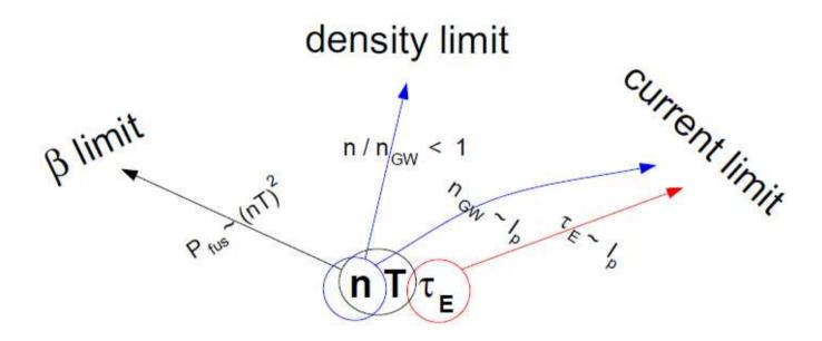
Optimising for Q=P<sub>fus</sub>/P<sub>ext</sub> drives operational point close to operational limits
