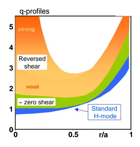
Hybrid operation aims at flat, elevated q-profile discharges with high q(0) Not clear if this projects to steady state, but it will be very long pulse...
