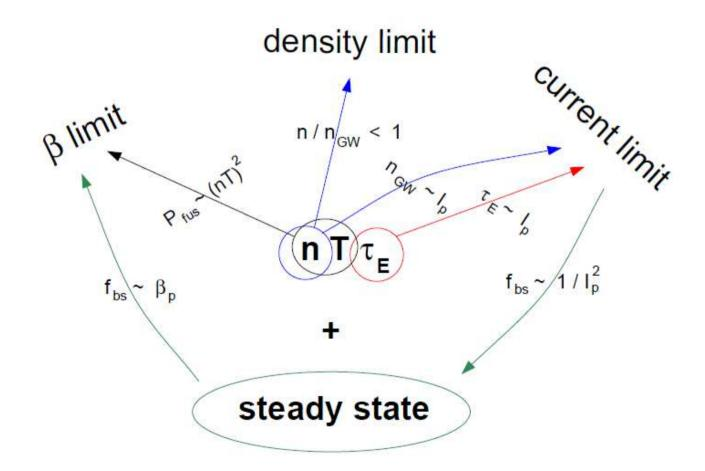
Including the steady state constraint emphasizes the  $\beta$ -limit (and de-emphasizes current limit)
