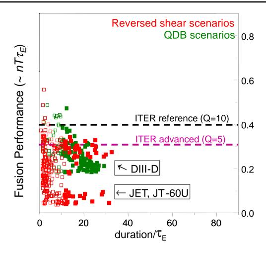
Good performance can only be kept for several confinement times, not stationary on the current diffusion time (10 – 50  $\tau_E$  in these devices)
