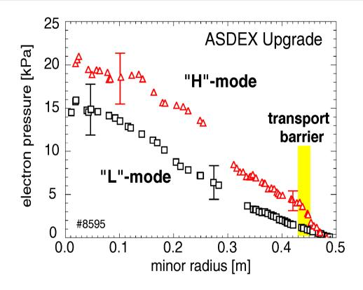
With hot (low collisionality) conditions, edge transport barrier develops
