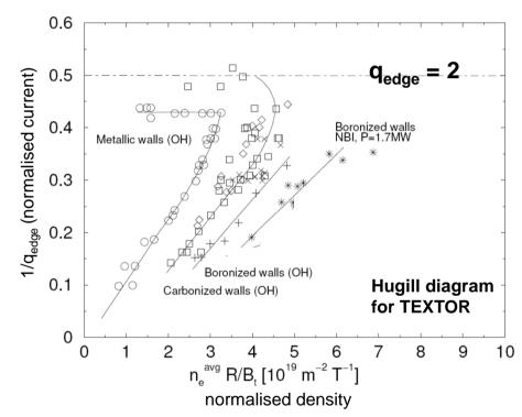
Limit to safety factor  $q \sim (r/R) (B_{tor}/B_{pol})$
