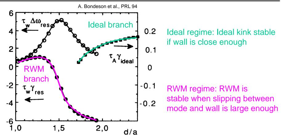
When ideal kink is wall stabilised, RWM can grow on wall time scale
