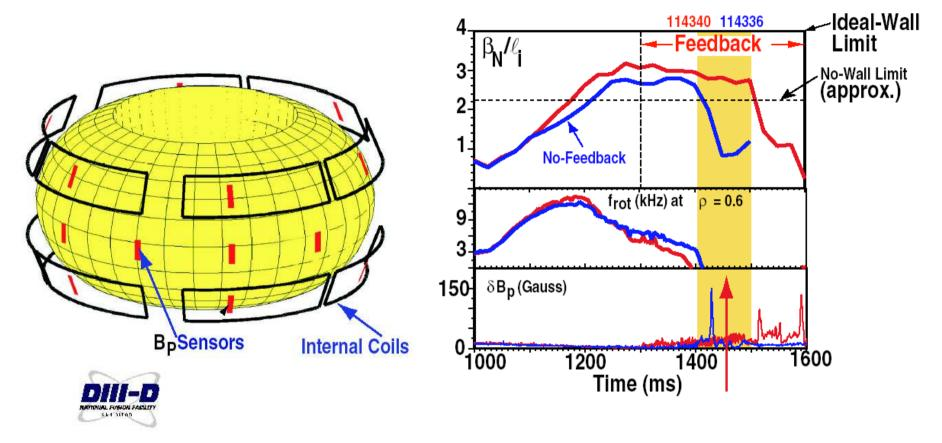
Feedback control using RMPs shows possibility to exceed no-wall  $\beta$ -limit
