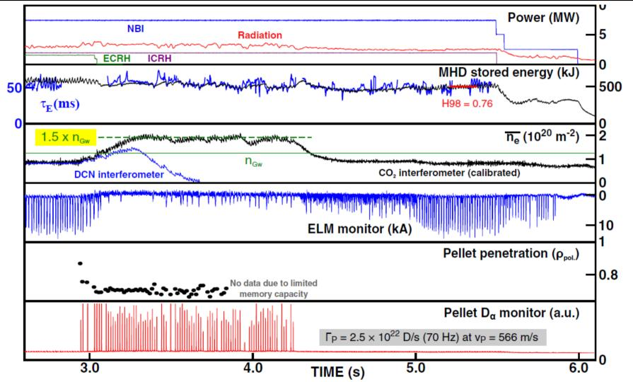
Stable operation at  $n/n_{GW} = 1.5$  using pellets
