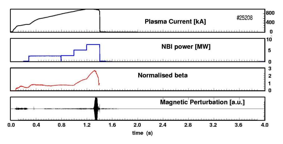
Target: a discharge that disrupts due to an early (2,1) NTM (q = 3.9,  $\beta_N$ =2.6)
