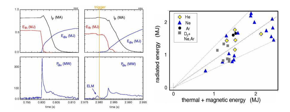
Reduction of power deposited on divertor measured by thermography
