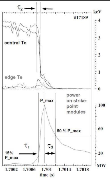
Typical timescale ≤ 1 ms, no clear variation with machine size, although tendency to increase...
